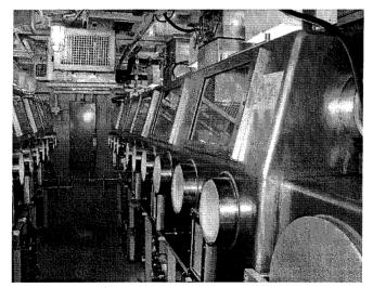
Figure 1 - Glove Boxes Inside the Mobile Plutonium Facility
